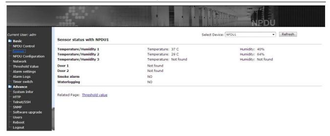
The above Sensor Monitoring Interface monitors the state of temperature/ humidity, Smoke, waterlogging and door open/close of the cabinets in which installed RPDU. When the temperature/humidity values exceed alarm threshold value, temperature/humidity value will become red and flash to alarm.
