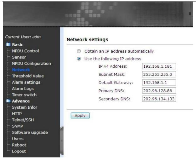
The above network configuration interface is used to configure RPDU network information. RPDU administrator can configure RPDU IP address, subnet mask, gateway address, DNS.
