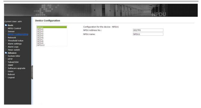
The above RPDU Device Configuration Interface is mainly used to configure daisy-chained RPDU's device, add or modify the daisy-chained device's name, address, interval-time for sequential power on, individual output unit's name and other information. Specific operations are as follows:
